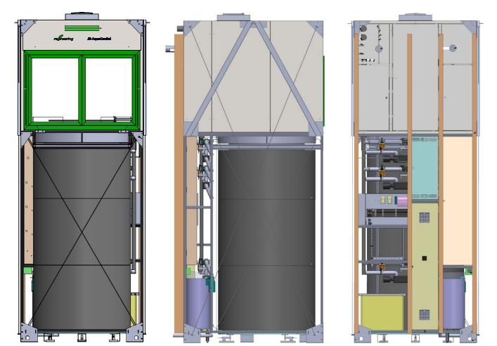
It integrates lysimeter, vegetation room, light, and climate chamber into a compact stand-alone solution. It is easily controlled with a tablet or remotely from your desk. Inputs are made via an intuitive user interface. Assemble your biotope of soil, plants, and fauna according to your needs and control the environmental parameters according to your research questions.
